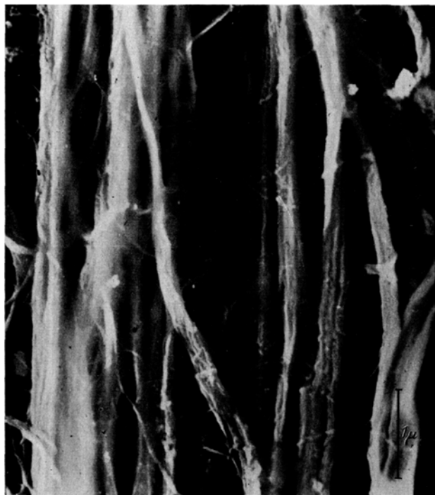
Fig. 5. — A section through a viscose fiber. Magnification 17,000 \times .
